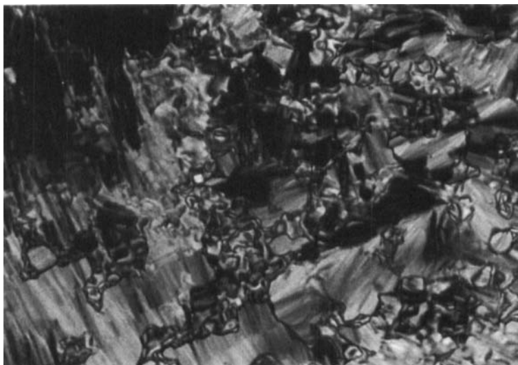
FIGURE 2. Optical texture of the lyotropic mesophase of 1e /chloroform mixture at 53°C, on heating, crossed polarizers, \times 100 . See Color Plate XXIV at the back of this issue.
